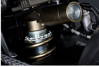
New piggy-back reservoir rear shock
